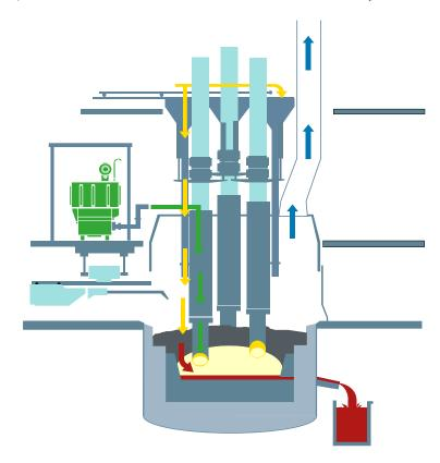
Figure 30: Submerged electric arc furnace (source: Elkem)
